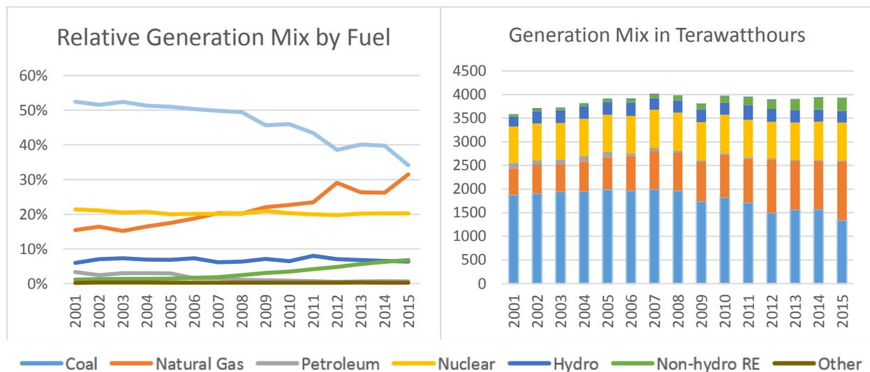
**Figure 27. U.S. Power Sector Generation Mix by Fuel, 2001-2015 (EIA).<sup>138</sup>** Coal’s share of power sector generation in the U.S. has fallen from 51.1 percent in 2005, to 34.2 percent in 2015. This trend is primarily driven by two forces: a market-driven shift from coal to natural gas in the U.S., and a policy- and technology-driven increase in the share of electricity generation from non-carbon sources, such as wind and solar.
