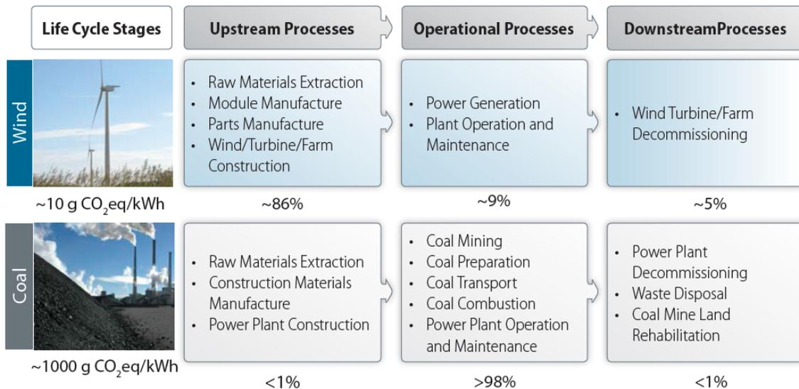
**Figure 17. Comparison of Life Cycle Processes and Greenhouse Gas Emissions for Wind and Coal Power by Life Cycle Stage.**<sup>88</sup> For fossil fuel generation, fuel combustion during operation emits the vast majority of GHGs. For renewable generation such as wind, most life cycle GHG emissions occur upstream of operation.
