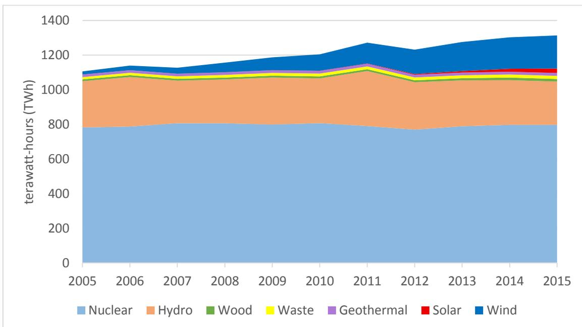
**Figure 29. Non-Fossil Fuel Electricity Generation in the U.S., 2005-2015 (EIA).<sup>146</sup>** Electricity generated from nuclear power and conventional hydropower in the U.S. has been fairly constant in the last ten years. Since 2005, most of the growth in electricity generation from low- and zero-emitting energy technologies in the U.S. is due to increased generation from wind and solar.
