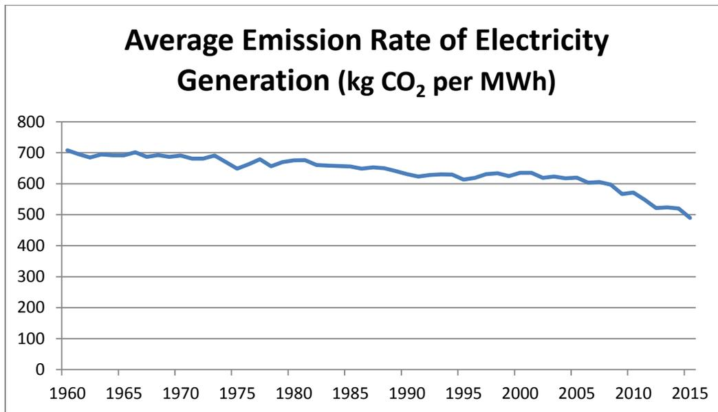
**Figure 26. Average Emission Rate of Electricity Generation in the U.S. Power Sector, 1960-2015 (EIA).<sup>137</sup>** The emission rate of the U.S. power sector is a key indicator of the climate impact of electricity generation, and varies significantly by fuel and technology. Between 2005 and 2015, the emission rate of U.S. electricity generation declined by 21 percent, primarily due to generation from coal being offset by increased generation from lower-emitting sources.
