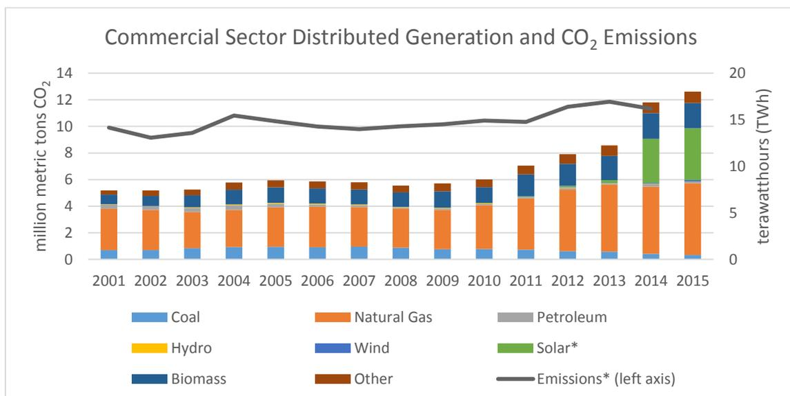
**Figure 15. Distributed Generation by Fuel and CO<sub>2</sub> Emissions from the U.S. Commercial Sector, 2001-2015 (EIA).**<sup>81 82</sup> The generation mix and subsequent emissions of distributed generation in the U.S. commercial sector differs significantly from the U.S. power sector generation mix. In 2013, the U.S. commercial sector generated 12.5 TWh of electricity, resulting in emissions of 11.9 MMT CO<sub>2</sub>.
