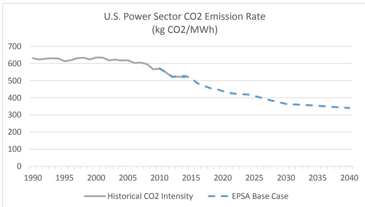
**Figure 31. CO<sub>2</sub> Emission Rate of the U.S. Power Sector, 1990-2040.**<sup>166 167</sup> Under current policies and measures, the CO<sub>2</sub> emission rate of the U.S. power sector is projected to continue its recent decline, reaching 340 kg CO<sub>2</sub>/MWh (750 lb CO<sub>2</sub>/MWh) in 2040.
