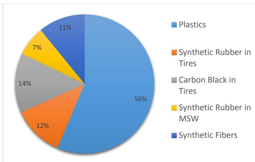
**Figure 9. CO<sub>2</sub> Emissions from Incineration of Non-Biogenic Waste in the U.S., by Source, 2014 (EPA).<sup>50</sup>** In 2014, incineration of non-biogenic waste accounted for 9.7 MMT CO<sub>2</sub>e, or 0.5 percent of total U.S. power sector GHG emissions.
