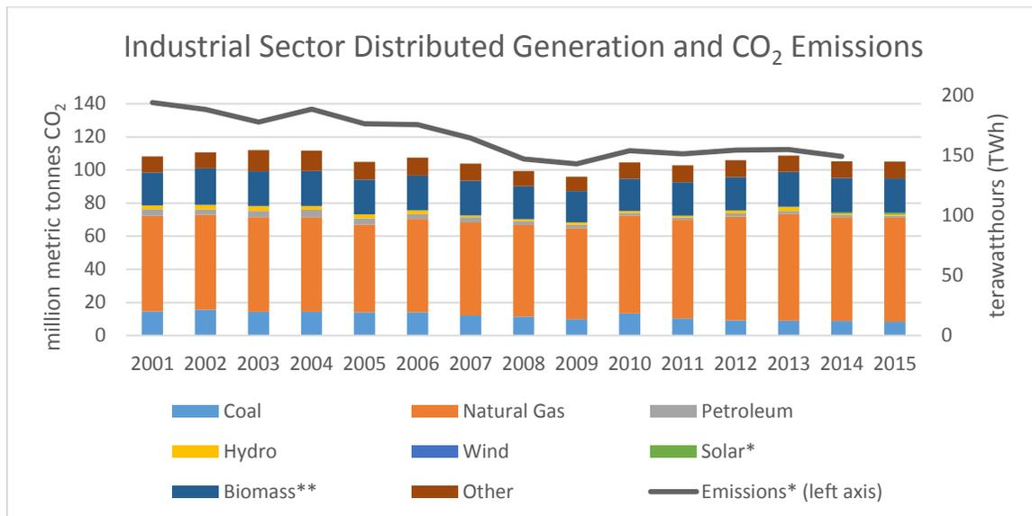
**Figure 14. Distributed Generation by Fuel and CO<sub>2</sub> Emissions from the U.S. Industrial Sector, 2001-2015 (EIA).**<sup>79 80</sup> The generation mix and subsequent emissions of distributed generation in the U.S. industrial sector differs significantly from the U.S. power sector generation mix. In 2013, the U.S. industrial sector generated 150 TWh of electricity, resulting in emissions of 112 MMT CO<sub>2</sub>.
