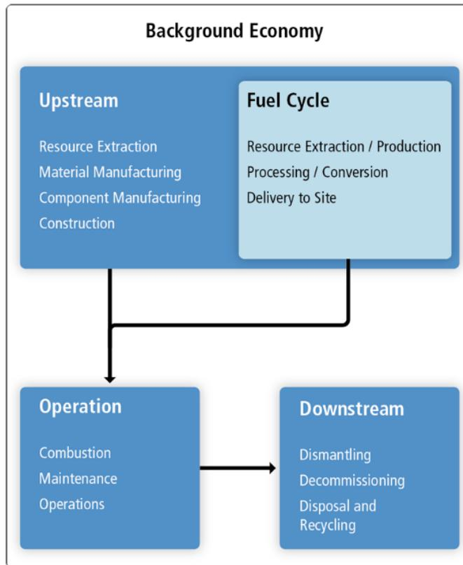
**Figure 16. Generalized Life Cycle Stages for Energy Technologies.**<sup>87</sup> The emissions attributed to the power sector in the *Inventory* include only “stack” or direct emissions from the combustion of fossil fuels. Additional emissions are associated with other stages in the full life cycle of an electricity generation technology.
