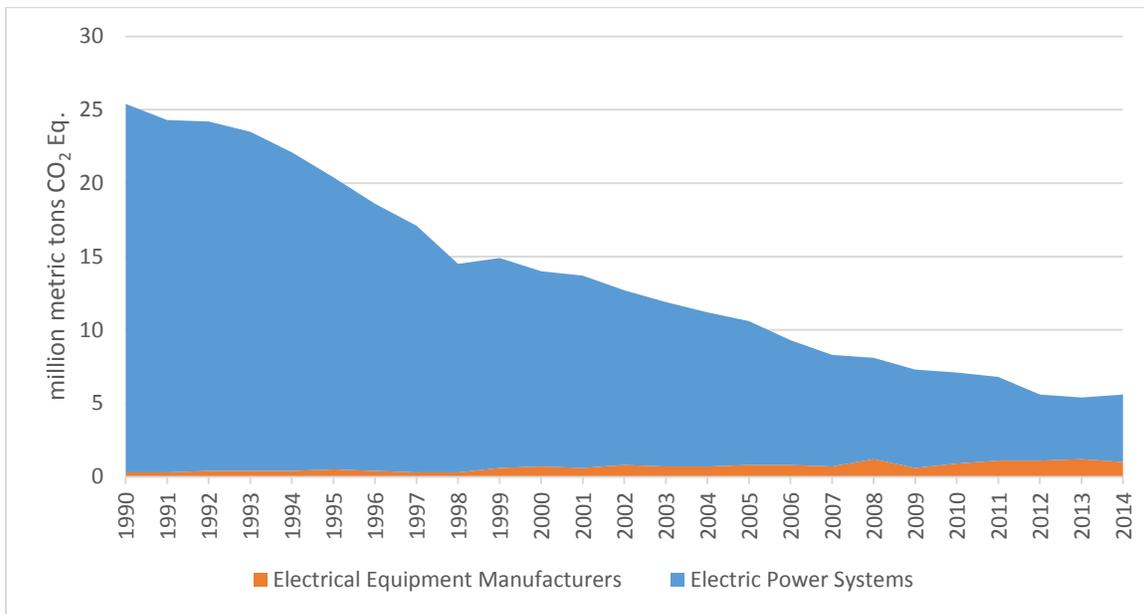
**Figure 10. SF<sub>6</sub> Emissions from Electricity Transmission and Distribution in the U.S., 1990 – 2014 (EPA).**<sup>58</sup> Emissions of sulfur hexafluoride (SF<sub>6</sub>) from equipment manufacturing and from electrical transmission and distribution systems in the U.S. decreased by 78 percent between 1990 and 2014.
