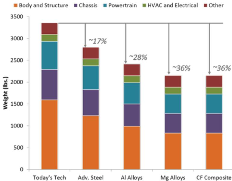
of Energy in conjunction with Magna International and Ford Motor Company demonstrated the potential for a 50% weight reduction through the use of multi-materials, although substantial reduction in content and function was required for this level of weight reduction.<sup>12</sup> Implementing multi-material solutions introduces an additional layer of technology challenges associated with multi-material joining, corrosion prevention, design tools, and performance predictions.
