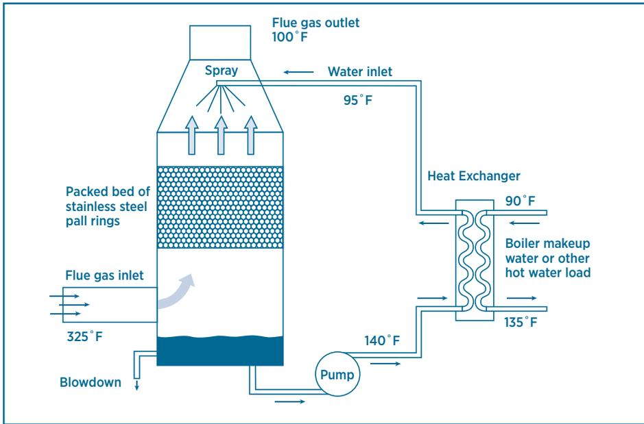
is supplied from blowdown heat recovery. The condensing economizer could also limit or decrease backpressure steam turbine energy production if the turbine discharge is used to balance a low-pressure header. The reduction in stack gas exit temperature reduces plume buoyancy and must be considered when modeling pollutant dispersion. Performance characteristics of both indirect and direct contact economizers are summarized in the table below.
