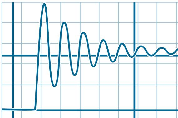
Figure 1. PWM pulse with reflected voltage or ringing
