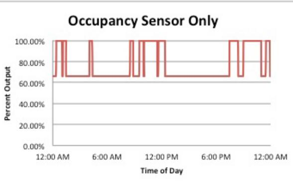
**Figure 12.** Monitoring for the same structure with an adjacent luminaire only controlled by an occupancy sensor. The sensor reduces the luminaire output by one-third after 20 minutes of no activity detection.
