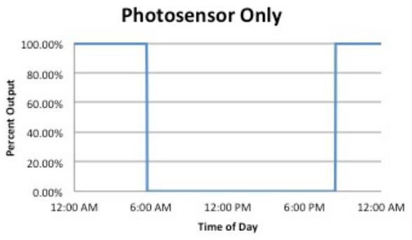
**Figure 11.** Real time monitoring for a mid-spring day of a luminaire in a parking structure only controlled by a photosensor. The luminaires turn on around sunrise and off around sunset.
