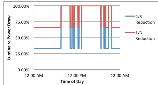
**Figure 15.** Sample data from an aboveground parking structure supporting an educational campus during the weekday. The figure depicts the usage when the low setting (when no activity is detected) is two-thirds and one-third full power. When the low setting is two-thirds reduction from full power, more energy is saved.
