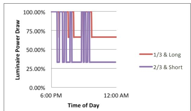
**Figure 17.** Sample data from an aboveground parking structure supporting an educational campus from 6:00 pm to midnight on a weekday. This graph compares little power reduction and a long time delay to a significant power reduction and a short time delay. Combining the short time delay with the greatest reduction in output permissible can optimize energy savings.
