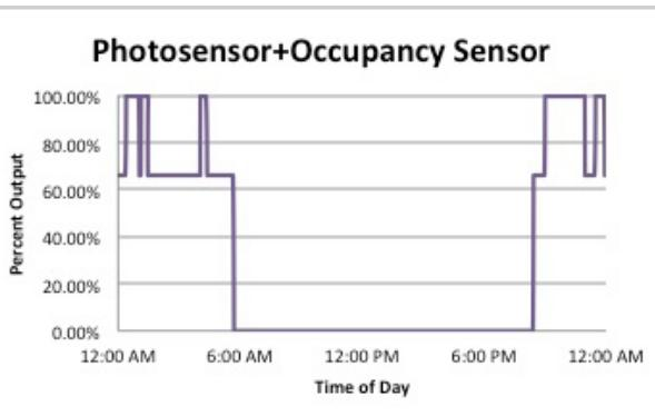
**Figure 13.** Monitoring for the same structure using both photo and occupancy sensor controls. When daylight is available, the luminaire is off. When it is dark outside, the luminaire is controlled by the occupancy sensor.
