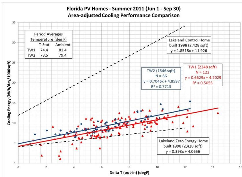
The cooling performance of the two TW homes is compared to a typical and a very high-performance home in Lakeland, FL. This method of comparing the cooling performance of different homes in different locations and periods was developed at FSEC (Chasar et. al. 2006 <http://www.ba-pirc.org/pubs/cooling/index.htm>) and is useful for visualizing comparative performance.
