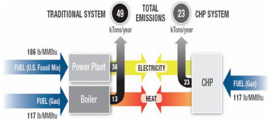
Figure 1. CHP Efficiency Conserves Fuel and Cuts Emissions (1)
