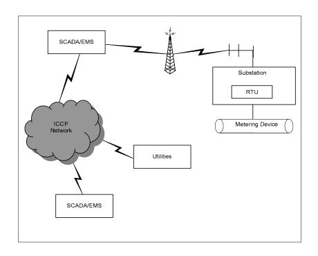
Measurements from metering devices on transmission equipment and in substations are collected by an RTU, which sends data to a utility SCADA/EMS system. ICCP network allows different utilities to share SCADA/EMS data.
