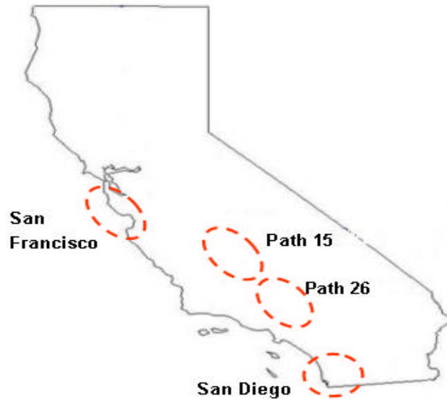
Figure 5 - CAISO Transmission Bottlenecks
