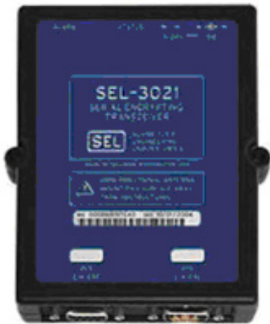
The CDC will be incorporated into a bump-in-the-wire link module, expanding SEL's current commercialized and FIPS 140-2-validated product line (SEL-3021) of serial cryptographic transceivers.
