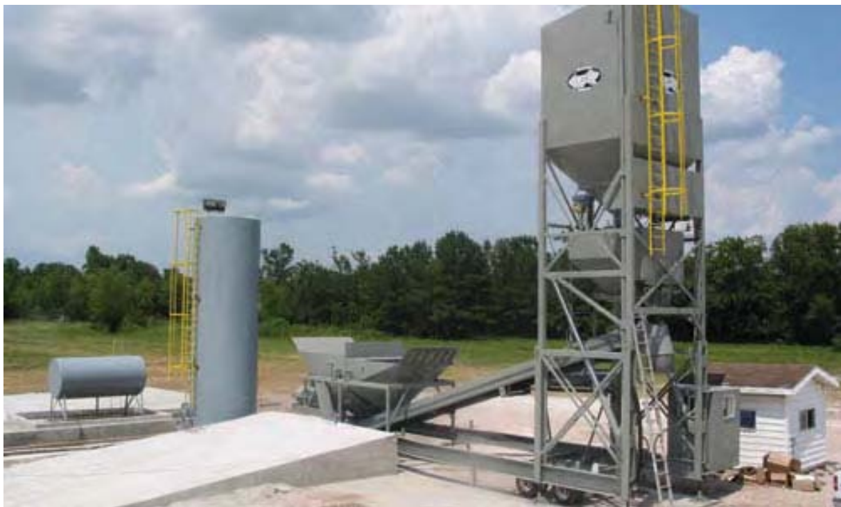
FIGURE 2.2-5 TYPICAL PORTABLE BATCH PLANT
