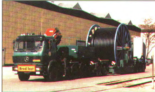
Figure 18. Special cable transport equipment
