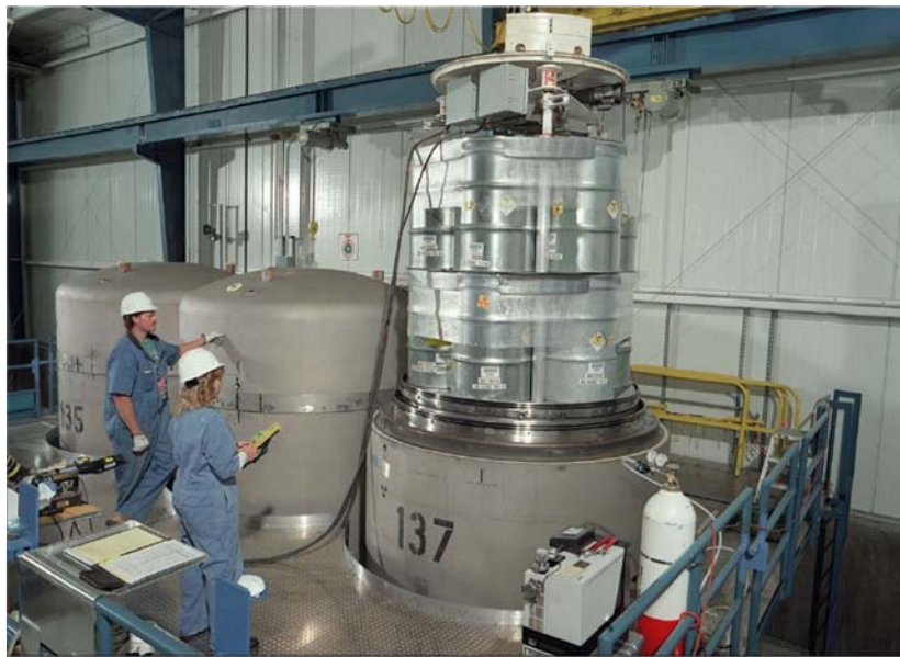
Figure S.12. Packaging of TRU Waste for Shipment to WIPP
