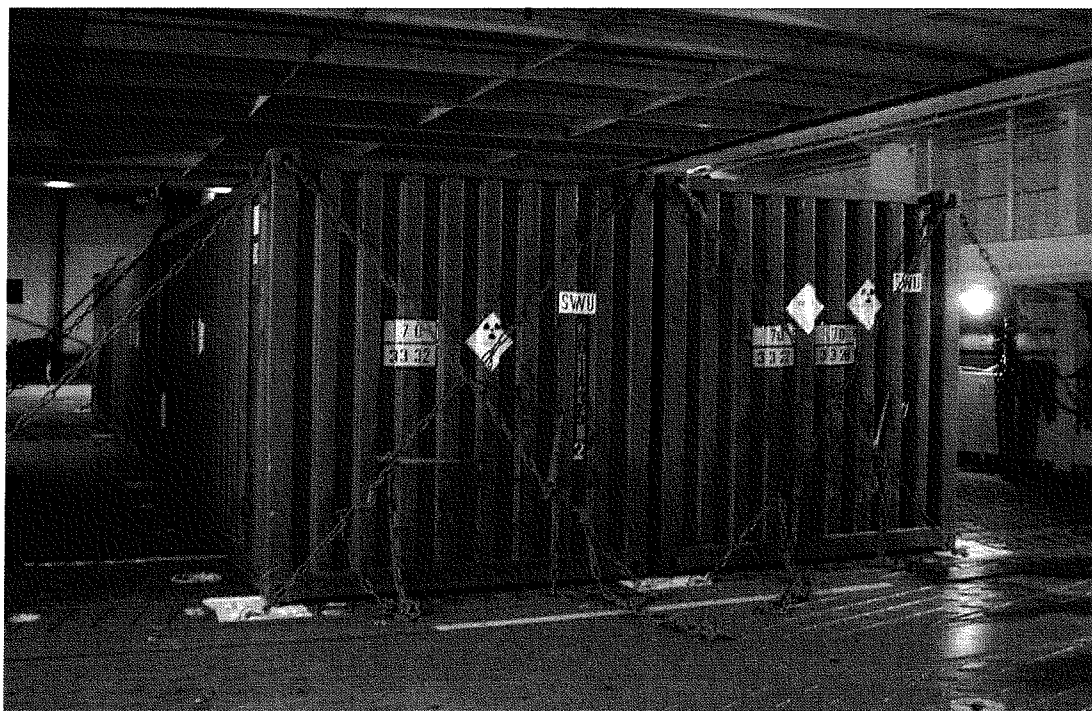
Figure 1–2 Nuclear Material in an ISO Container Secured within the Hold of a Ship
