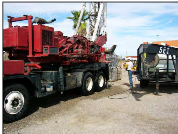
Photograph 2-6 Example of a Auger Rig
