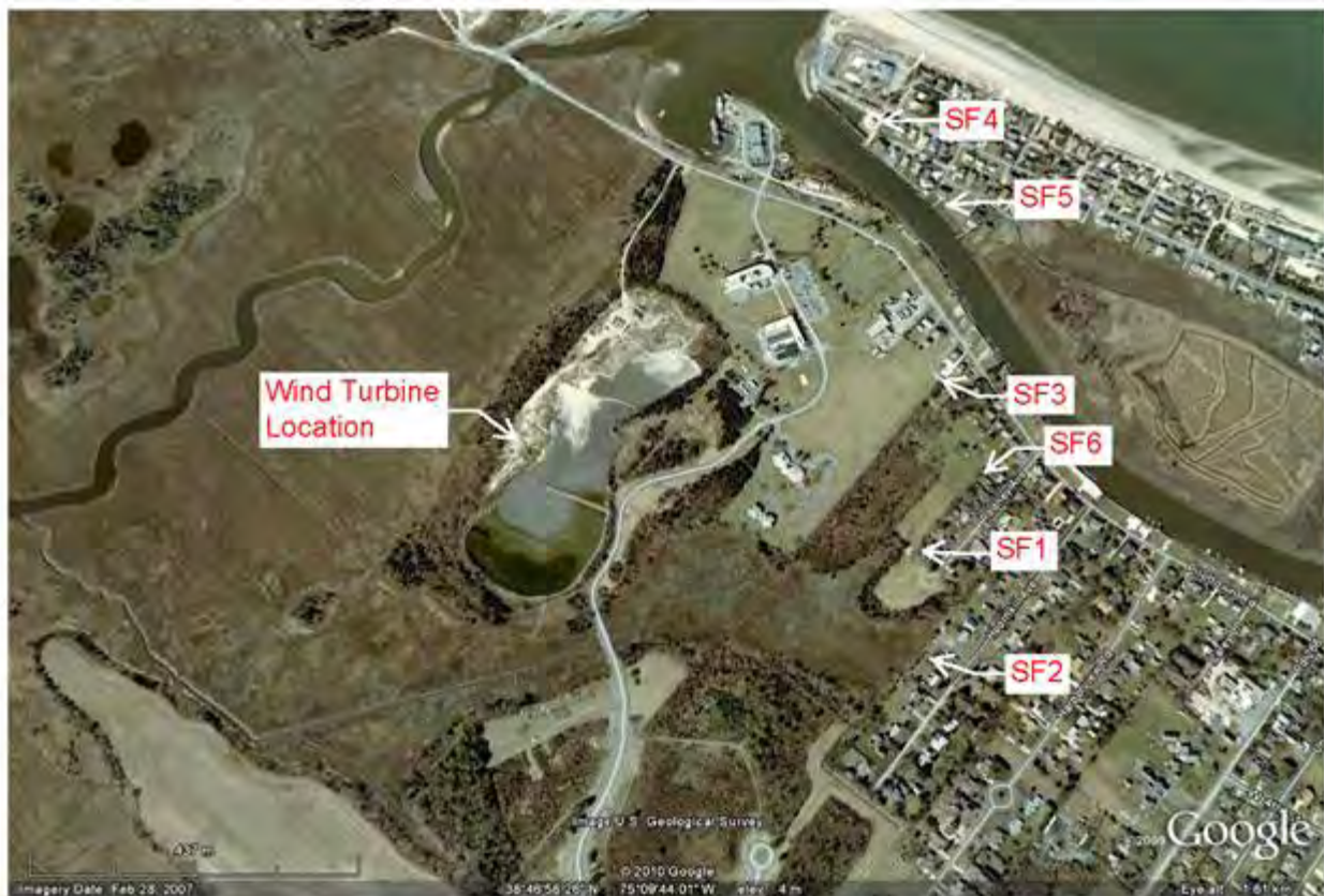
Figure 3-7. Aerial photograph with shadow flicker (SF) analysis locations identified by number.
