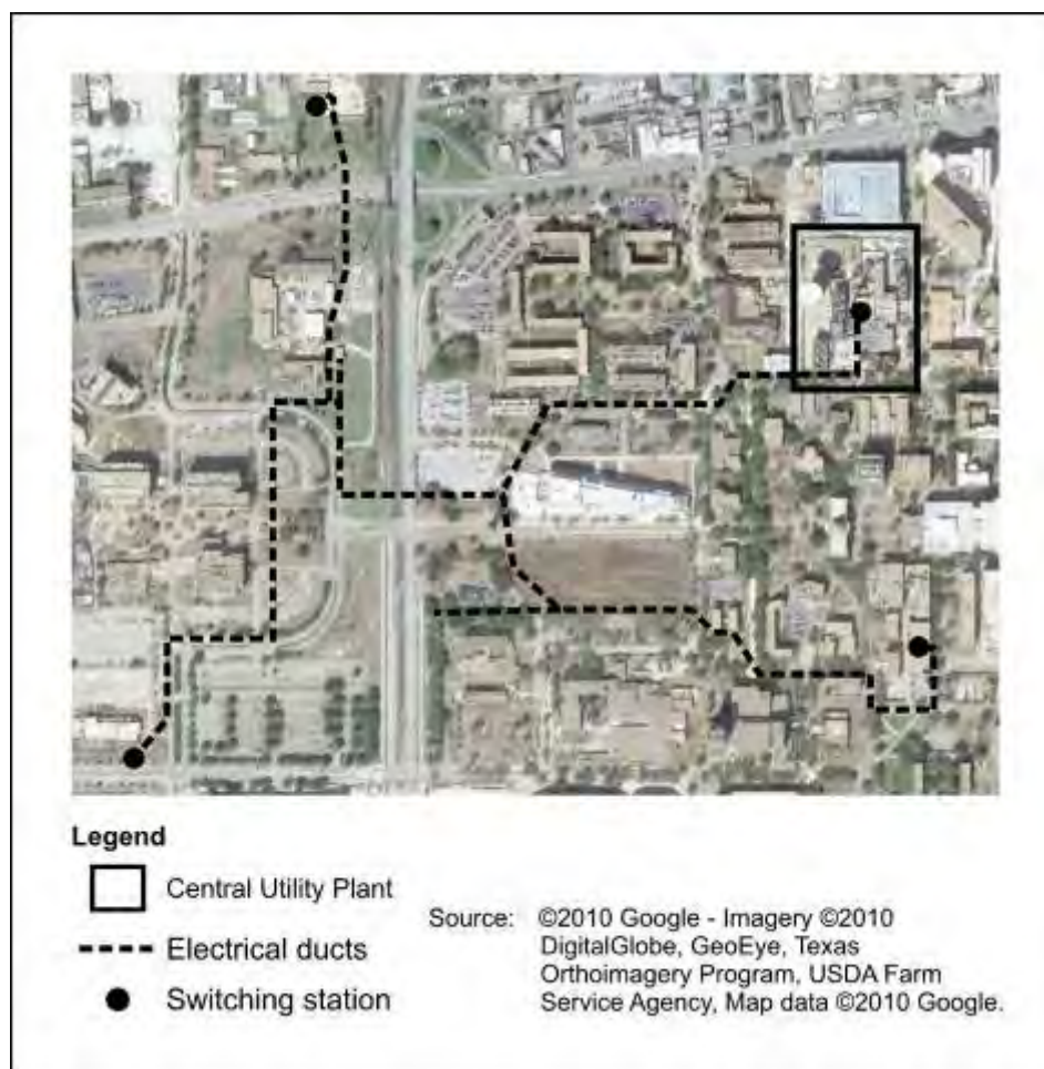
Figure 2-3. Approximate routes of electrical ducts and locations of switching stations.
