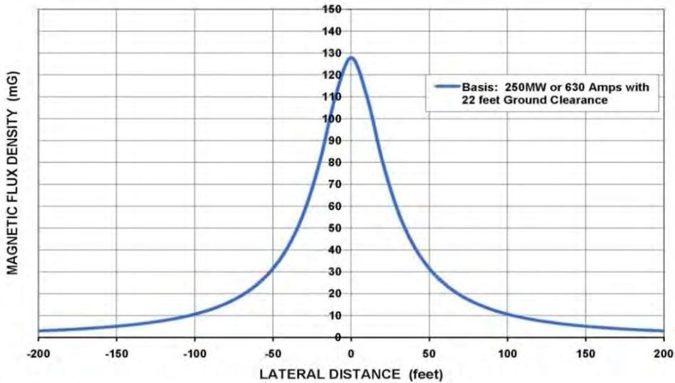
Calculated per IEEE Standard 644 at 1.0 meter (3.28 ft) above ground.
