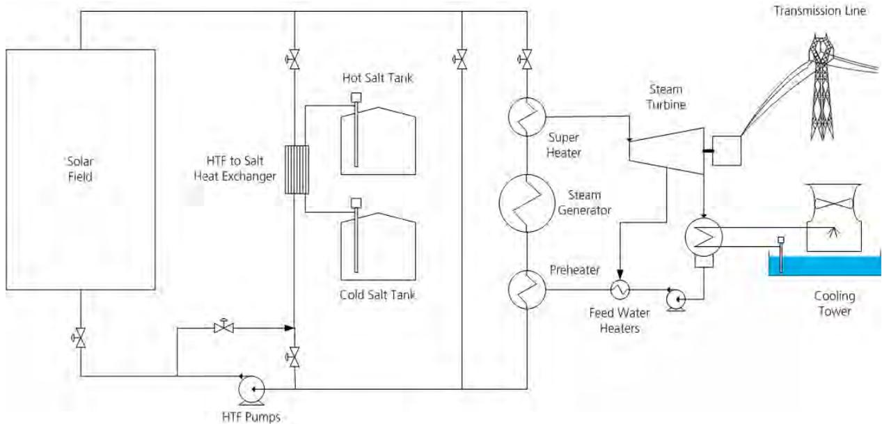
Figure 2-4 Thermal Energy Storage System
