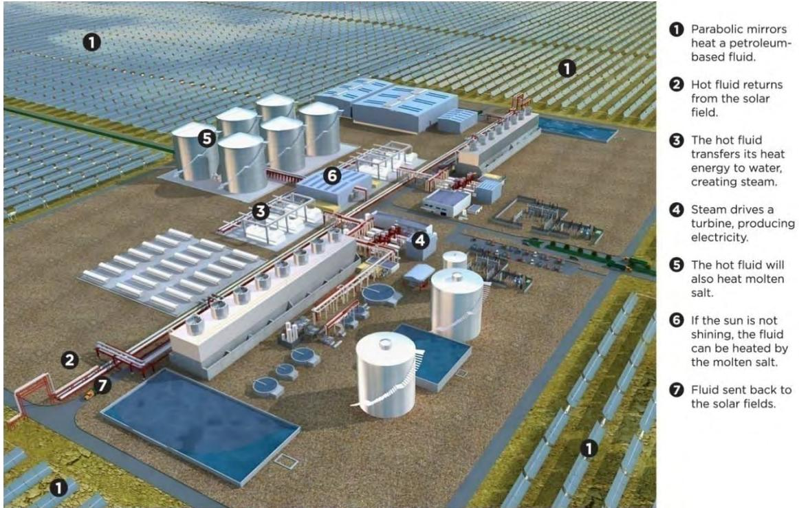
Figure 2-3 Solana Generating Station Diagram
