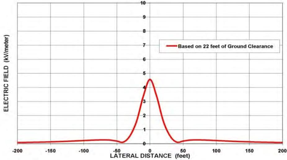
Calculated per IEEE Standard 644 at 1.0 meter (3.28 ft) above ground.
