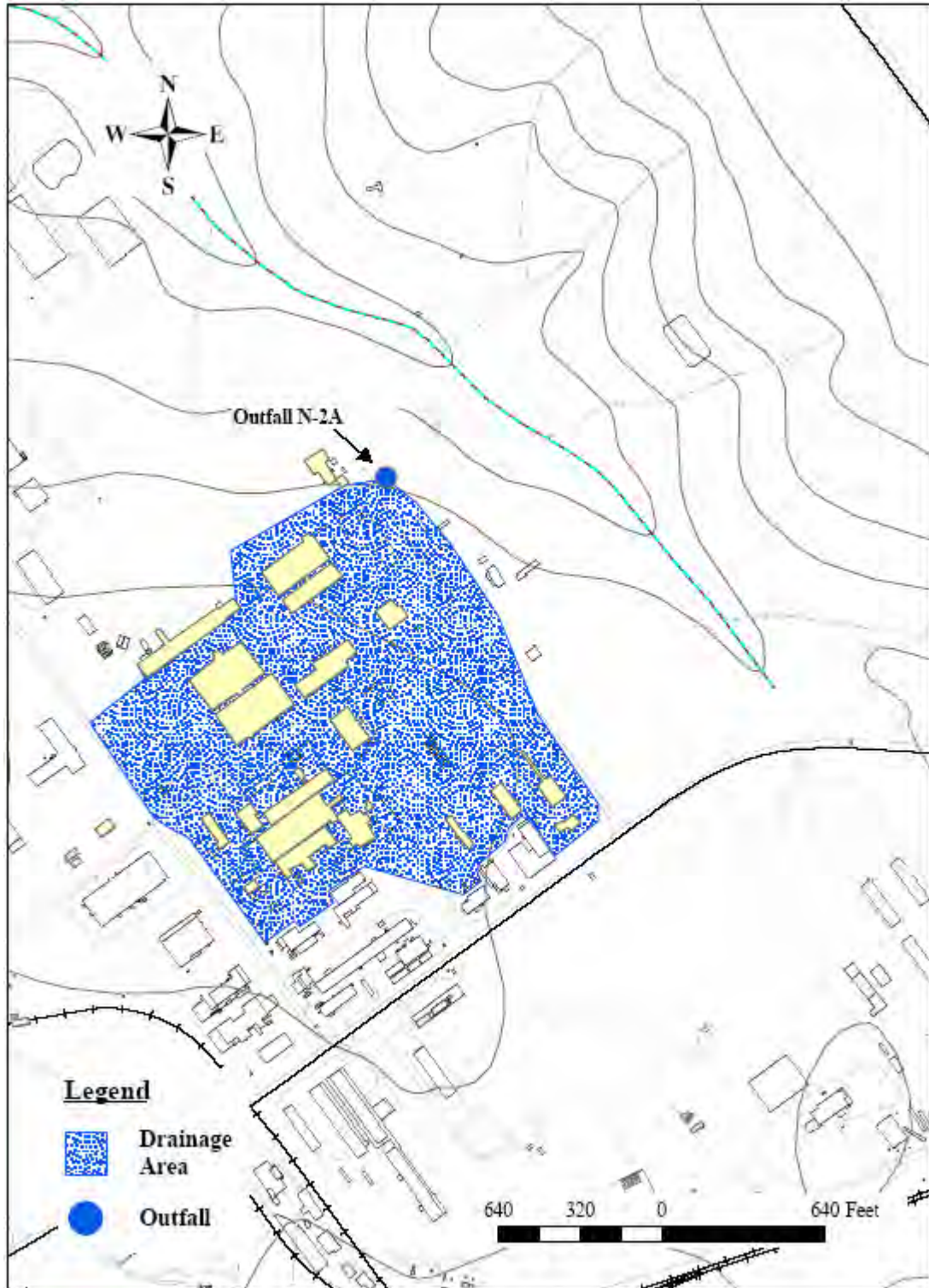
Figure 2-77. Location of Stormwater Outfall N-2A and Associated Drainage Area.
