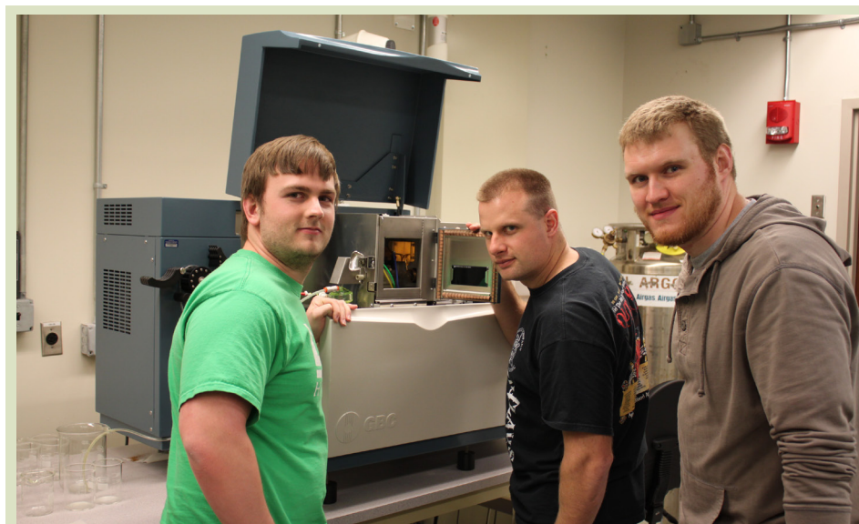
Figure 1. UT graduate students Joshua Chandler, Captain Joshua Molgaard (U.S. Army), and Matt Cook working on the UT inductively coupled plasma-time of flight mass spectrometer, which is used to analyze gas-phase separations.
