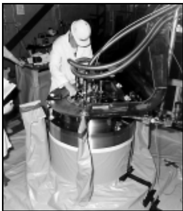
Nuclear chemical operator attaching hoses to ports in the top of a multi-canister overpack holding 290-300 irradiated fuel assemblies from Hanford's K Basins, in the cold vacuum drying facility, Hanford Site
