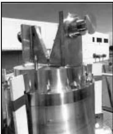
Spent fuel shipment cask for moving spent fuel from K Basins to new canister storage building, Hanford Site, Richland, Washington
