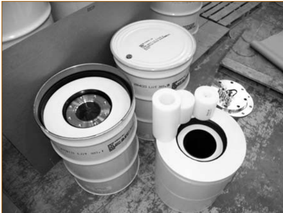
Example of containers used to store Transuranic Waste.
