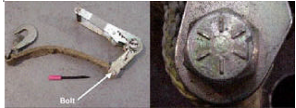
Ratchet Tie-Down and Suspect/Counterfeit Bolt
