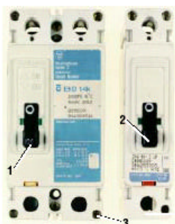
Suspect/Counterfeit Circuit Breaker (factory seals missing, amperage not stamped on toggle switch, epoxy filler missing)
