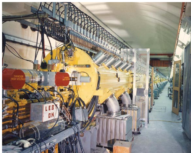
The 200 MeV proton linear accelerator at Brookhaven National Laboratory is used for high energy physics research and isotope production.
