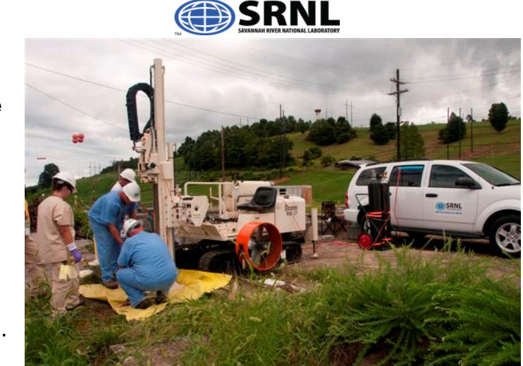
and demonstrate an economical, minimally-invasive tool for characterizing elemental mercury source **zones** in the subsurface by adapting existing technology for a unique application.
