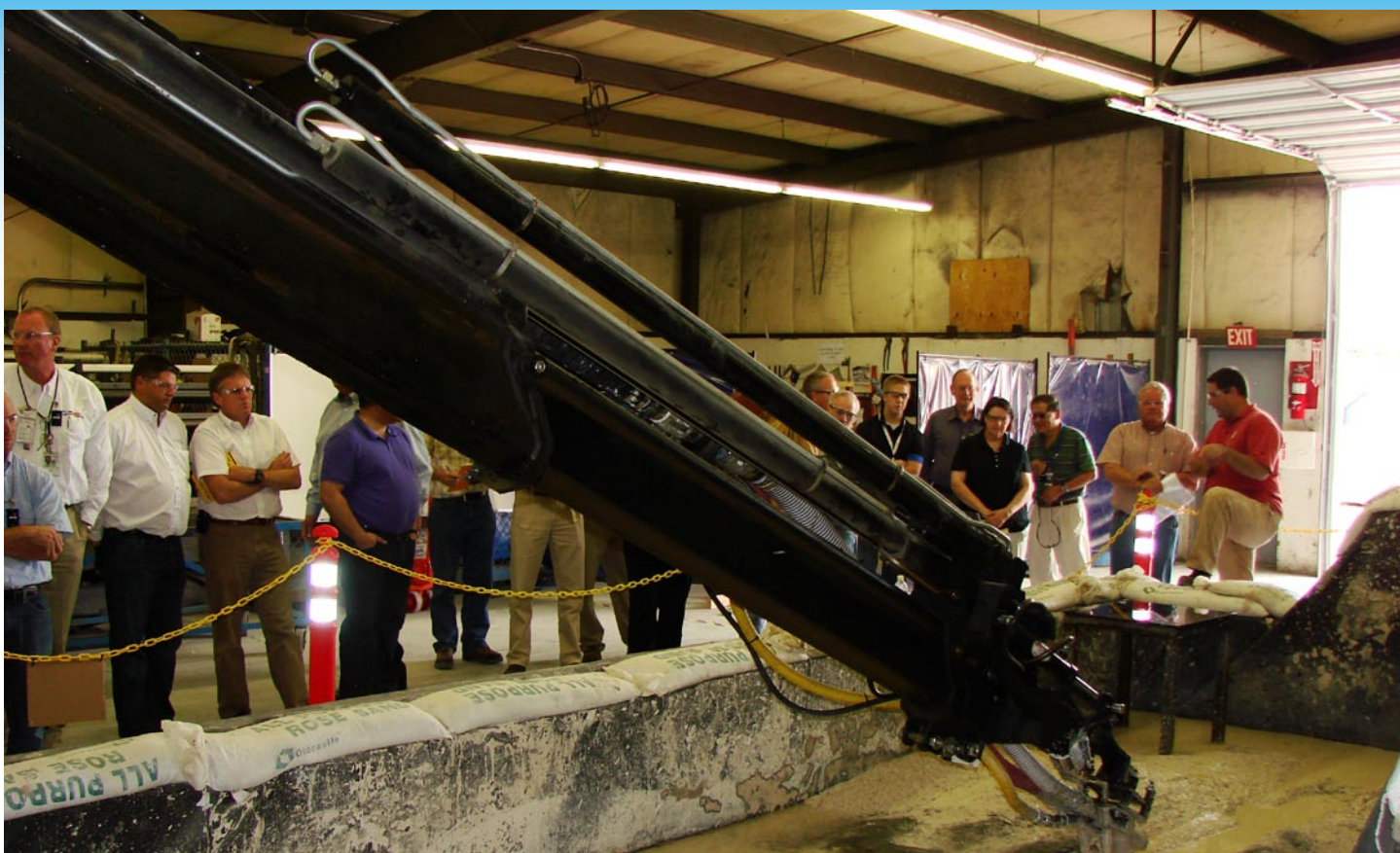
Engineers conduct a demonstration of the Mobile Arm Retrieval System's vacuum retrieval system for staff members at the Office of River Protection at Hanford. The Recovery Act-funded technology is expected to improve tank waste retrieval at Hanford.
