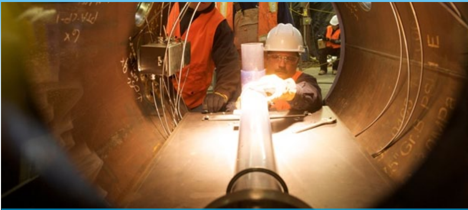
Engineers prepare a mockup of the Experimental Breeder Reactor II's internal parts for a test run.
