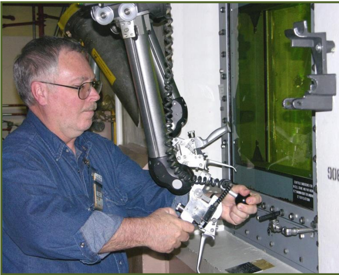
Perry concentrates on operating a robotic manipulator arm at the CPP-659 hot cell, where he was trained for several months before moving to CPP-666.
