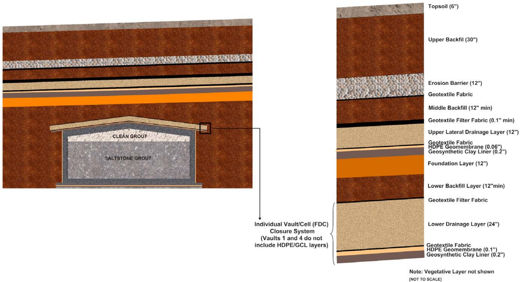
Figure 3.2-20: Saltstone Disposal Facility Conceptual Closure Cap Layers
