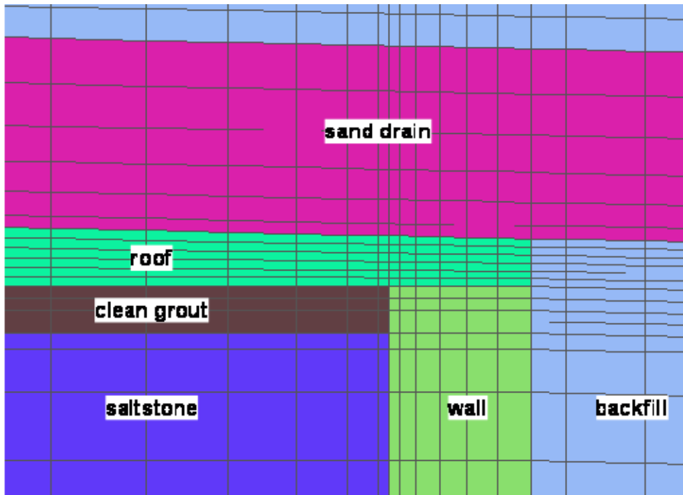
Figure 4.4-22: Vault 1 Upper Corner Detail for PORFLOW Vadose Zone Modeling
