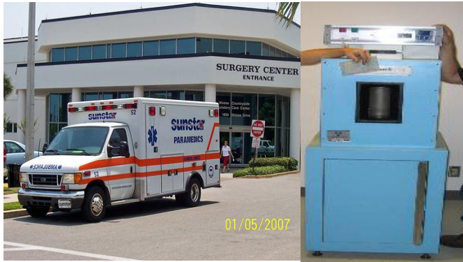
A self-shielded cesium-137 irradiator used to irradiate blood products and prevent a deadly transfusion disease (graft-versus-host disease)
