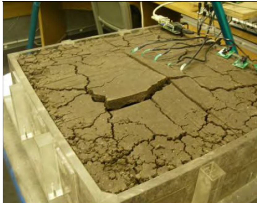
Figure 46. Surface curling in clay mass after 2 days.
