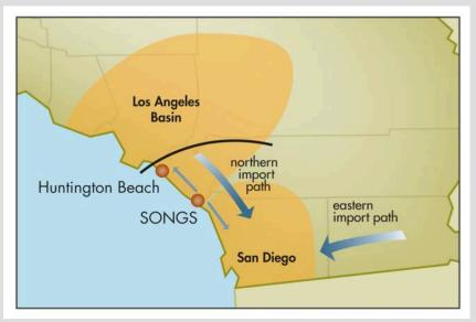
Recent completion of the Sunrise Powerlink transmission project in the SD area, however, has had unanticipated reliability benefits, by making the area less dependent on its two pre-existing high-voltage transmission connections with external supply sources.
