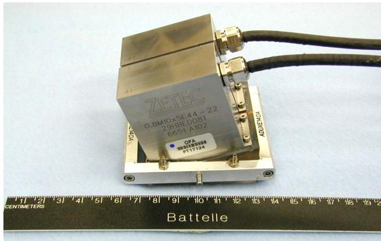
**Figure 5.4.** Photograph of PA-UT Probe
