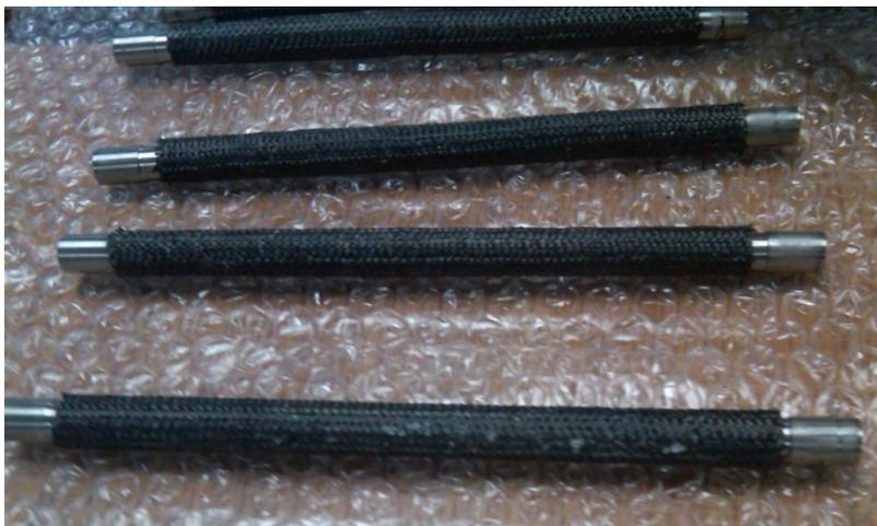
Figure 13. Silicon carbide clad test rodlets.
