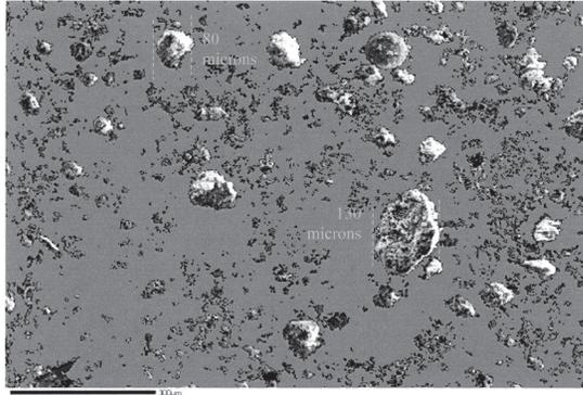
Fig. 2. Micrograph of HTF solids. A fraction between 75 and 150 microns is 37 vol% is often used in the PCT, but the entire FBSR solids was encapsulated and evaluated as PCT and TCLP.
