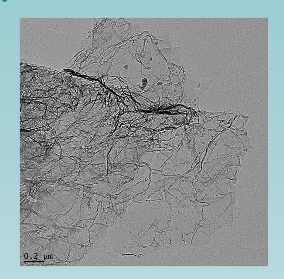
■ We evaluated graphene in Li-O<sub>2</sub> cells containing a typical liquid electrolyte
