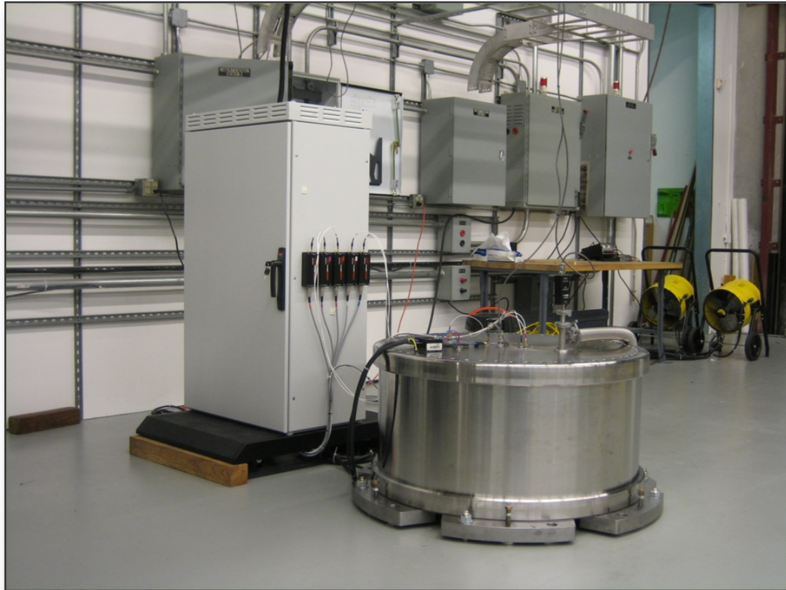
Generation One: Prototype 20 kW | 5 kWh Flywheel System
