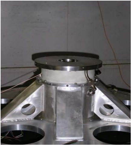
HTS Stability Bearing Cryostat Installed in DOE 5 kWh Flywheel
