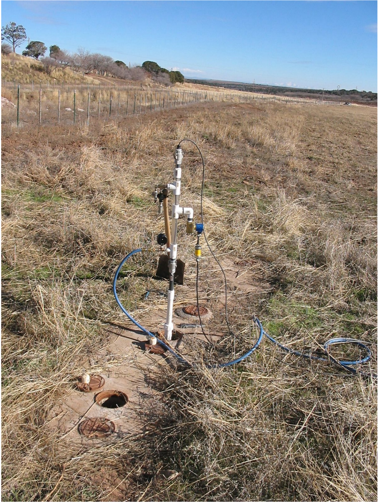
Figure 4. Pneumatic Slug Test Well-head Apparatus
