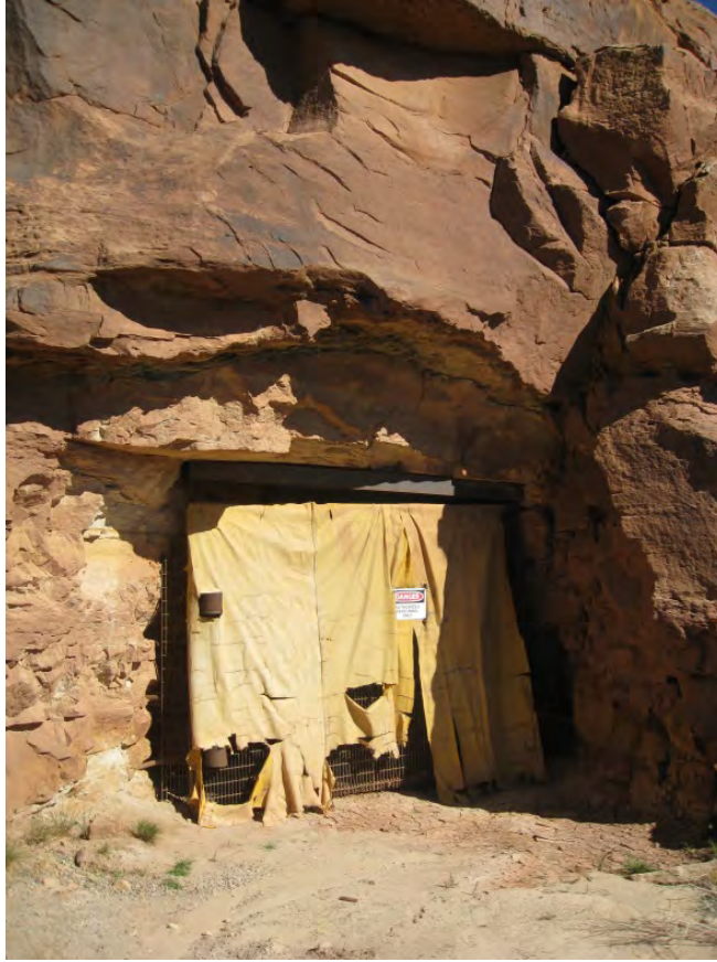
FIGURE 3.12-8 View of Entrance to Underground Mine at Lease Tract 18 (The Cotter Mine entrance has a locked gate to prevent unauthorized entrance and is covered with fabric to control ventilation.)
