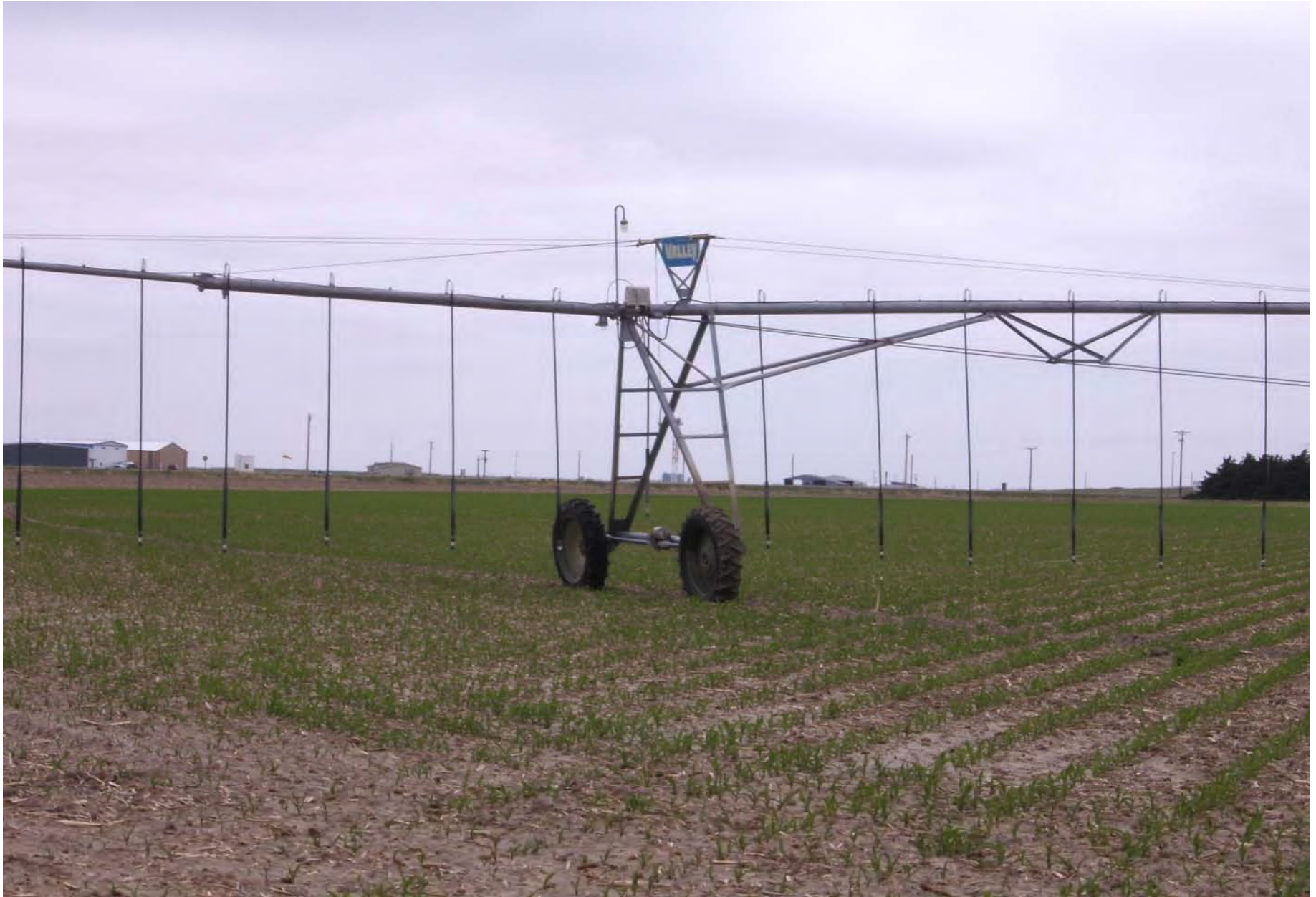
22. Section of a center pivot irrigation system
