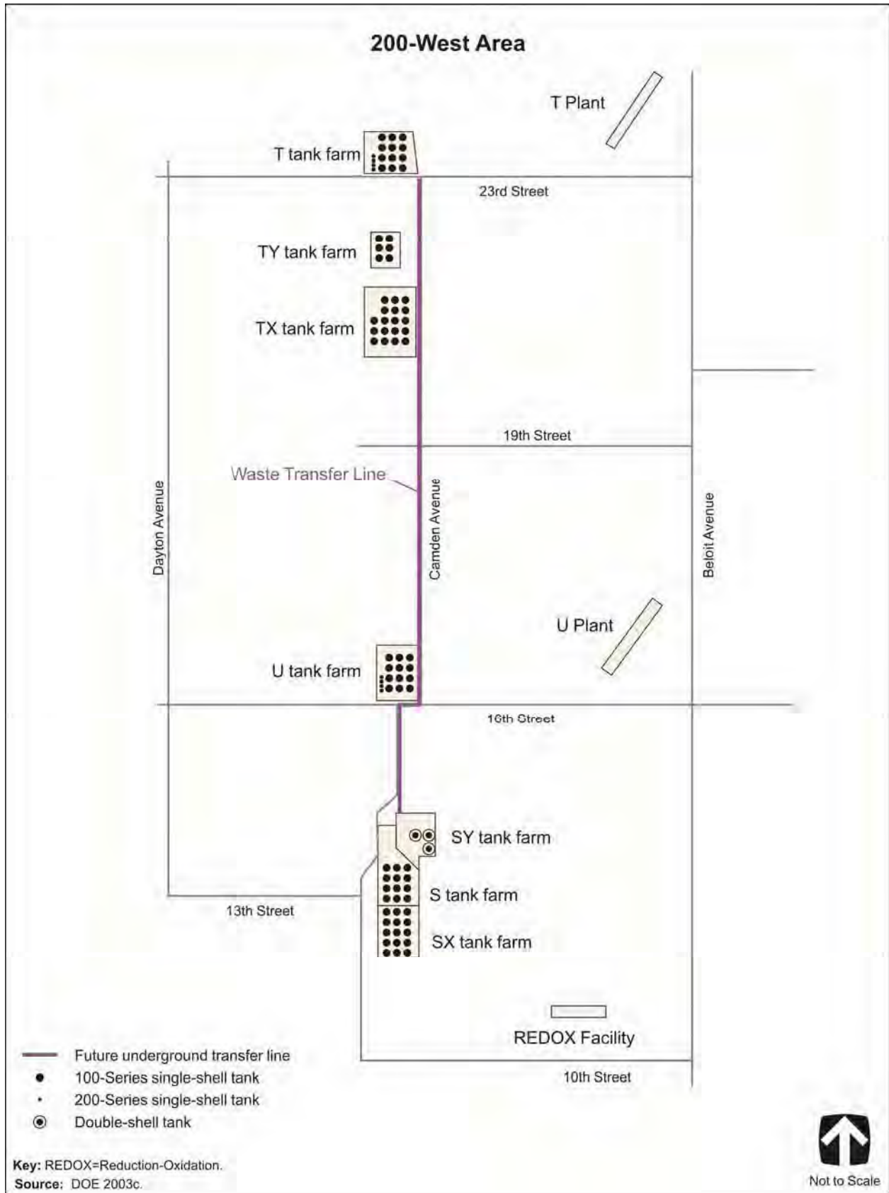
Figure E-7. Future 200-West Area Underground Transfer Line
