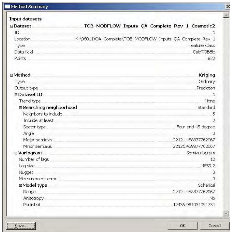
Figure L-8. Screen Print of Default Settings From Top of Basalt Surface Interpolation Using ArcGIS Geostatistical Analyst
