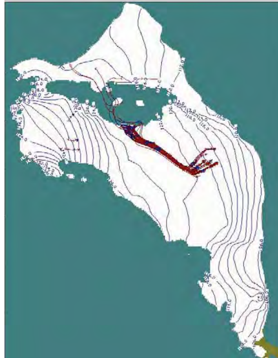
Figure L-94. Hydrogen-3 (Tritium) Plume Pathline Analysis Run 195 (root mean square error = 2.056 meters) – Selected as Alternate Case Flow Model
