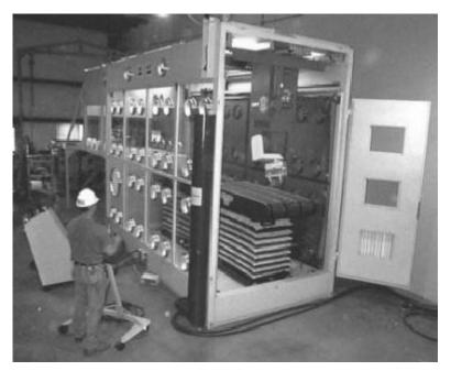
Figure I–20 Example of a Remotely Operated Dismantling System and Inspection Station
