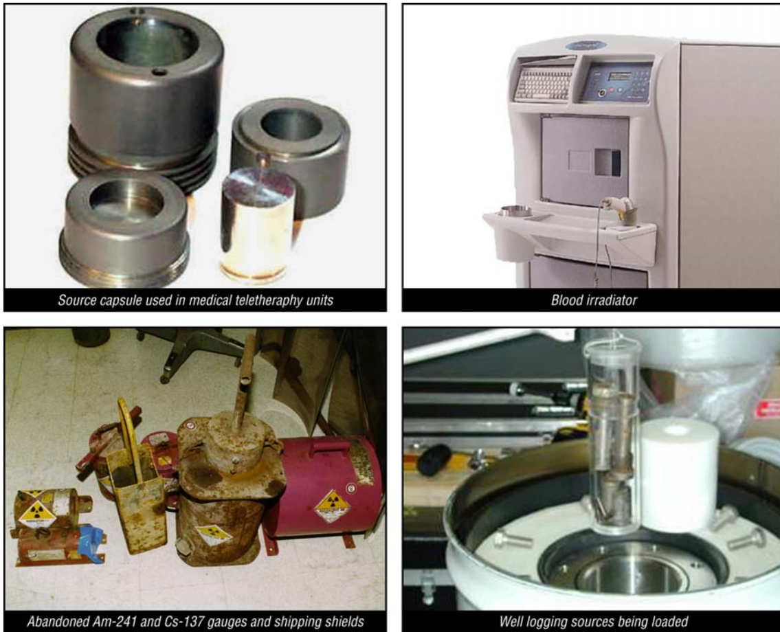
Abandoned Am-241 and Cs-137 gauges and shipping shields
