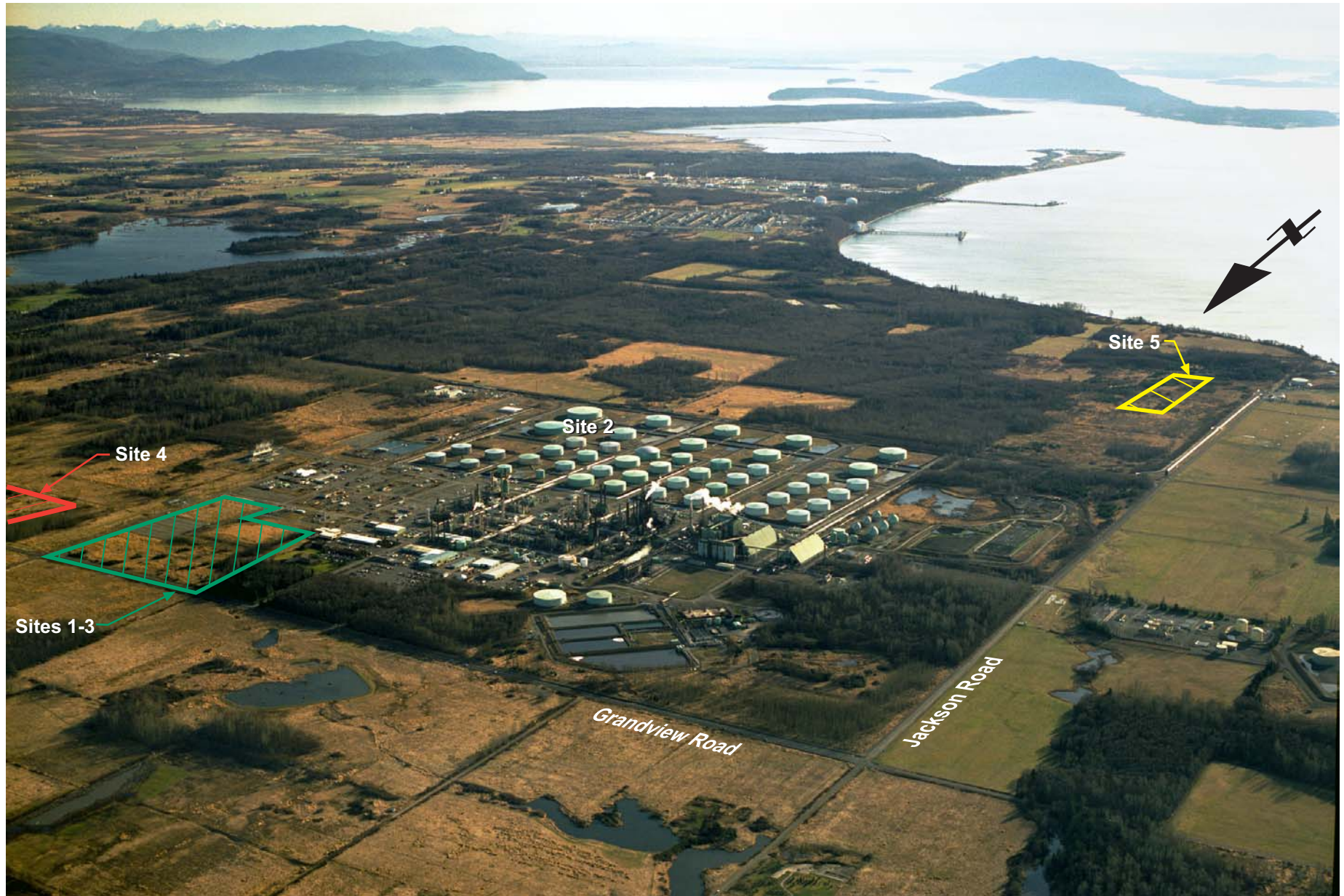
FIGURE 1-7 PREFERRED AND ALTERNATIVE CONSTRUCTION LAYDOWN (STAGING AND ASSEMBLY) AREAS BP/CHERRY POINT/WA
