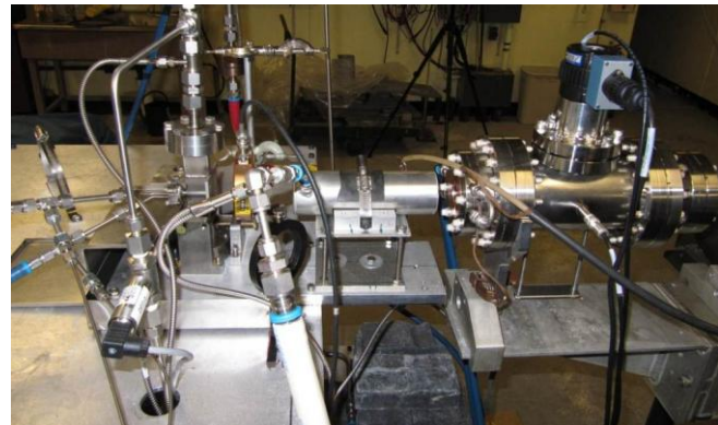
Figure 2-9. Molybdenum Target Testing Setup at Argonne National Laboratory
