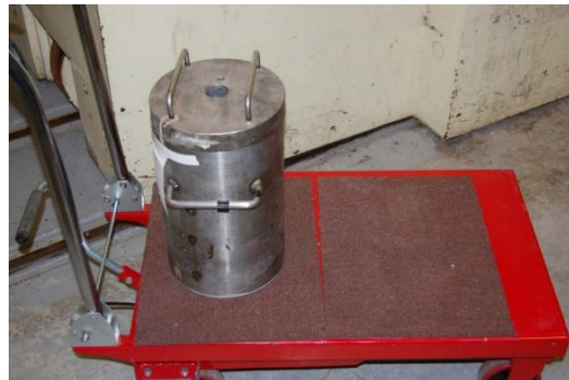
Figure 2-10. Lead Transport “Pig” Container Used to Move the Irradiated Molybdenum Targets
