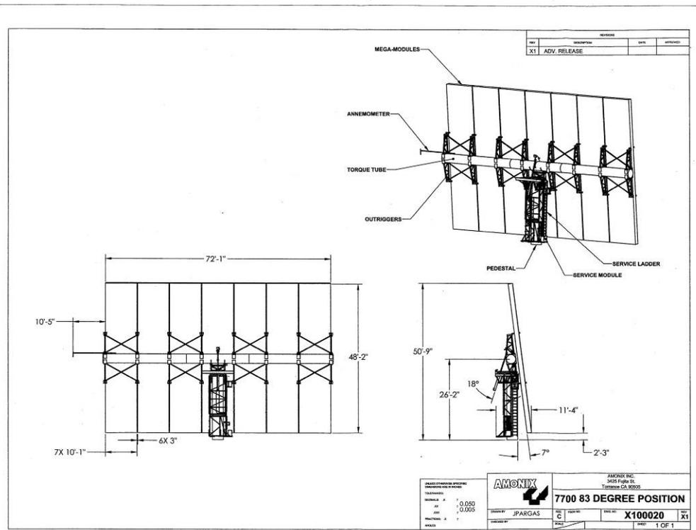
Figure 5. Amonix Specification Drawing – 83 Degree Position
