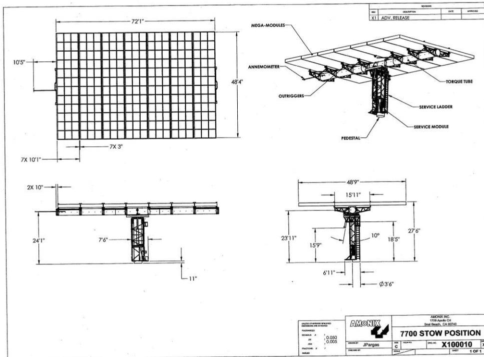
Figure 4. Amonix Specification Drawing – Stow Position
