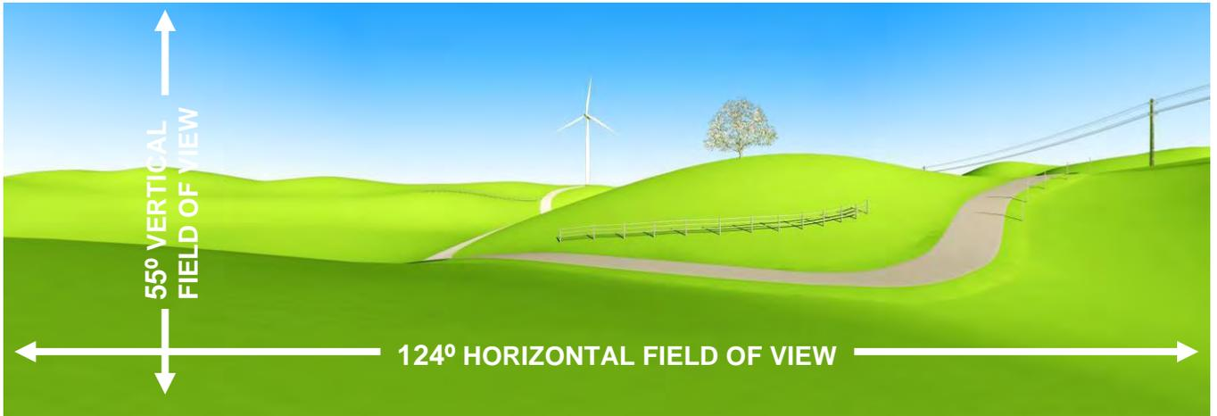
In order to correctly place existing objects that are in front of the 3D model of the development, these foreground objects are overlaid, from the original photograph, onto the computer generated image using photo shop software.
