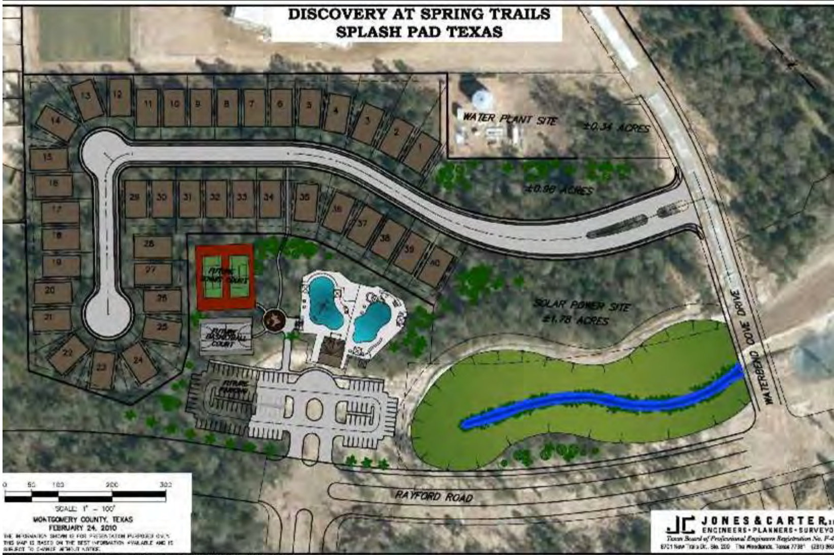
Figure 2-3. Detailed view (artist’s rendering) of the location where the solar farm and battery would be constructed, which is adjacent to the community recreation area. (From the center of the figure, north is toward the upper left corner.)
