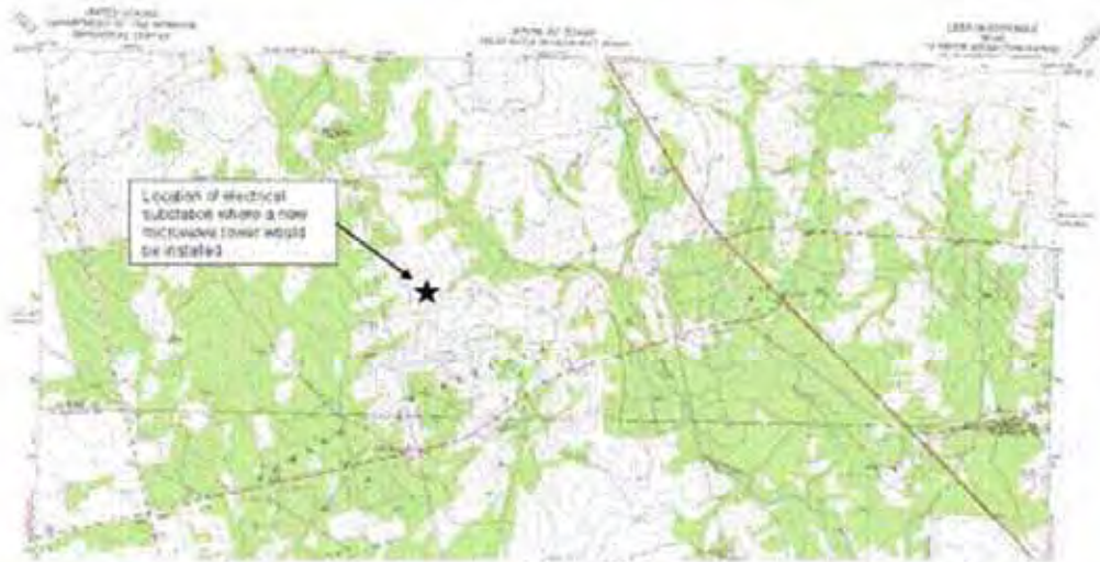
Figure 2-3. Clip from USGS 7.5 minute quadrangle map, Lees, Texas, showing the location in Howard County where there is now a substation and where a new microwave tower would be installed under the CCET project.
